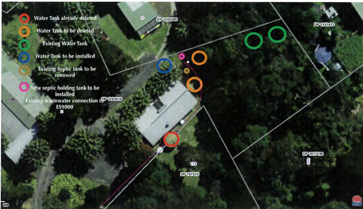
Figure 4. Location of current building footprint with notes on items needing to be moved.
